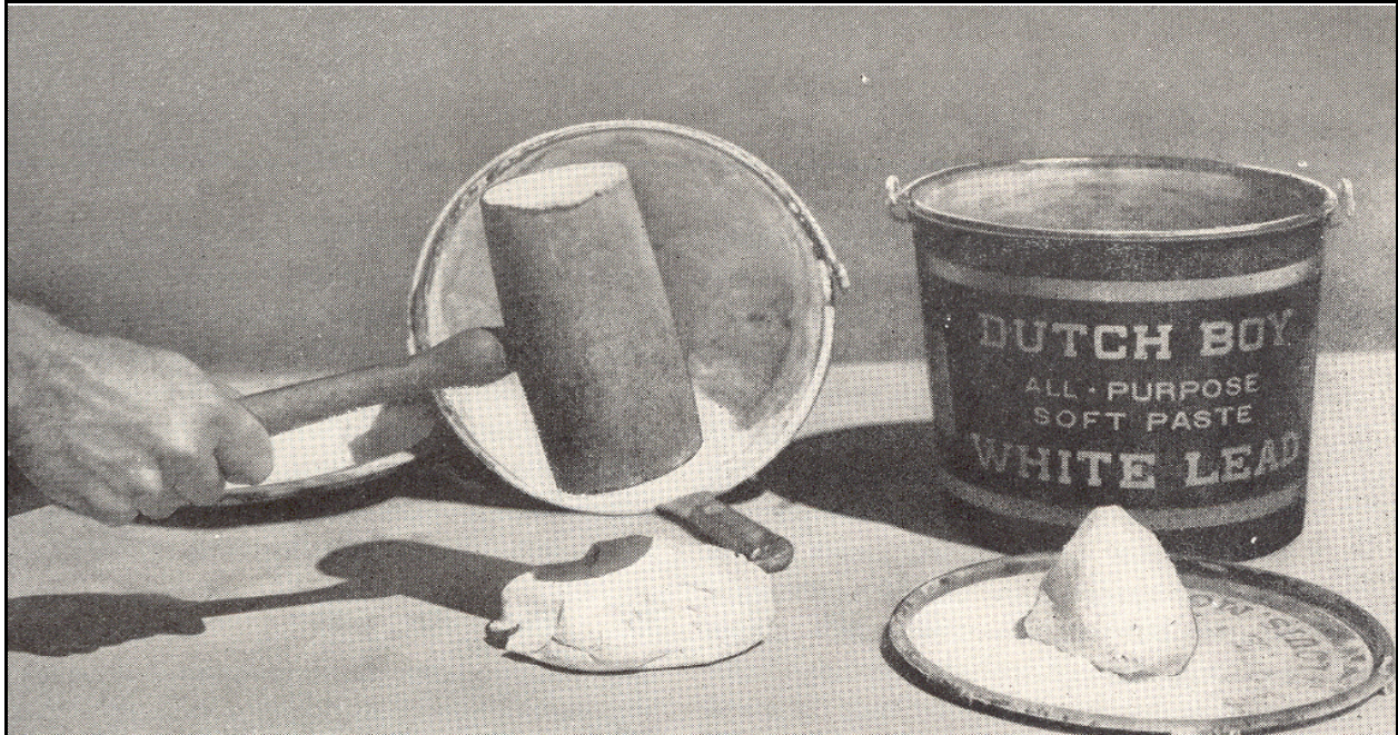
Figure 106: The ILO 1921 Geneva Convention prohibited the use of white lead unless it was in the form of a ready made paint. The use of the paint paste shown here, could give rise to dust which exacerbated lead exposure. Image from Dutch boy Painter Magazine , Vol. 31, 6, 1938. P. 128..
